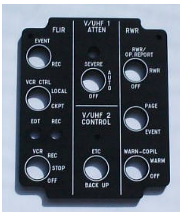
UHF Control panel
